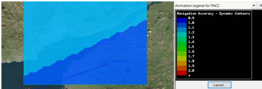
Figure 9. Contours of GPS accuracy in meters
