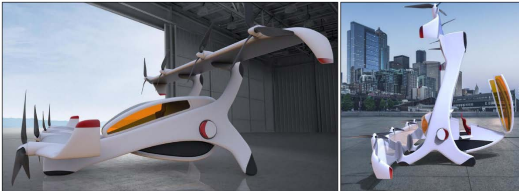
Figure 4. Neoptera's eOpter in horizontal flight (left) and parking (right) configurations
